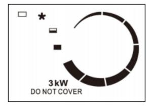
LEFT Dial: Used to select the desired setting. (fan only, fan and one heating element, fan and two heating elements).
