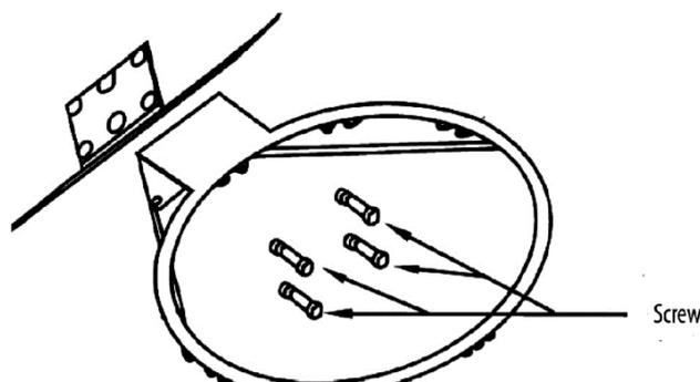
2. Once inserted with the hoop attached, the bolts should be tightened which will cause them to expand inside the holes and lock into place. Next, fit the net to the hoop by hanging it onto the metal hooks.
