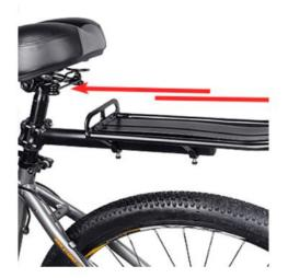
4. Push forward or backward to adjust to the desired position
