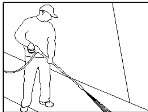
Figure 6-Optimum Angle to Cleaning Surface
