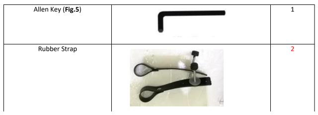
Please note, bolts may come screwed into the ends of the X-Brace. Using the Allen key provided ensure that all bolts are removed before assembly.
