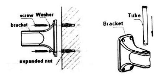
To mount the bracket to a wall drill four M8 holes to match the holes located in the mounting bracket. Secure the bracket to the wall using the provided screws and expanding nuts.
