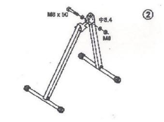
Now, join part C with part A; ensuring that the holes align. Fasten with the larger bolt, washer and nut. Part F are now the legs and should be on the ground.
