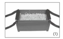
3. Place the top screen on top as show and squeeze out as much water as possible, using the handles to push firmly down on the wet material. If the material packs down too far, add more material to fill the space and repeat.
