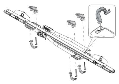
3. Attach the locking straps to the carrier.
