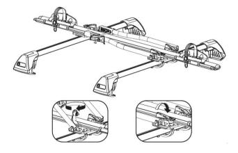
7. Once the carrier is in place, remove the key and check that it is securely installed. Strap the front wheels to the carrier and fix the support arm onto the frame of the bike.
