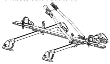
5. Adjust the clamps according to the roof rails, ensuring that the bike carrier is mounted centrally.
