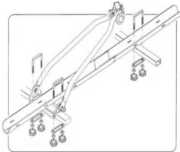
Attach the carrier to the roof bars using the U-shaped bolt, spacers and nuts.
