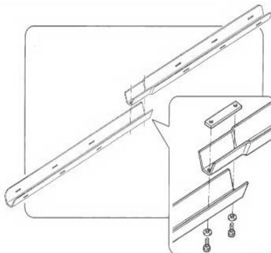
Attach the support bars together using the attachment plate and 2 nuts and bolts.
