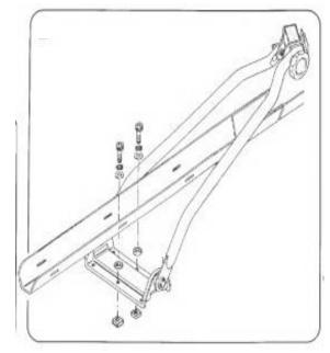
Attach the bicycle holder to the support bars using 2 bolts, nuts, washers and 4 spacers.
