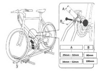
Attach the support clamp to the frame of the bike. For a frame of diameter 29-32mm, use the 80mm bolt to secure. For a frame of diameter 34-52mm, use the 100mm bolt to secure.
