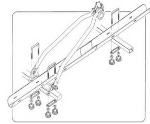
Attach the carrier to the roof bars using the U-shaped bolt, spacers and nuts.
