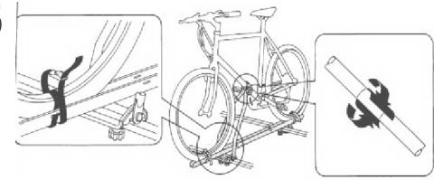
Secure the bike to the carrier by strapping down the front and back wheels. Please see diagram above to help. Ensure tightly secure before departure.
