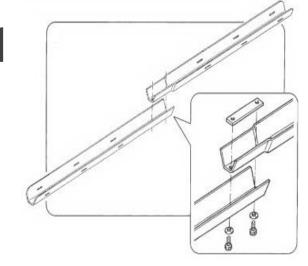
Attach the support bars together using the attachment plate and 2 nuts and bolts.
