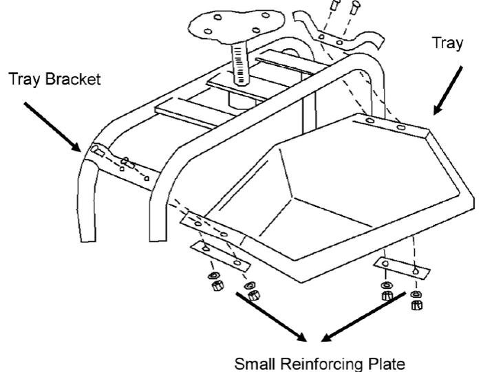
4. Attach the seat to the seat post which is located on the top of the frame. Line up the holes in the seat and the seat post and insert a medium screw through each of the four holes in the top of the seat. Ensure that they also go through the seat post holes and secure on the underside with a medium washer and a medium nut on each screw.
