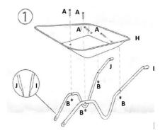
**1.** Grab the barrow tub (H) and attach it onto the support bars (I, J) using four bolts (A). To secure this, place four screw caps (B) over the end of the screws.
