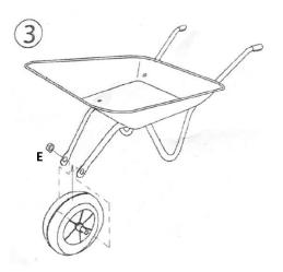
**3.** Secure the screw (C) using one nut (E). Tighten this to secure the product together alongside all other nuts. Make sure to not over tighten the nuts.
