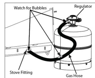
1. Prepare a soapy water solution (one part washing up liquid to three parts water) to test for gas leaks in the connections. Apply a generous amount of the soapy mixture to the regulator assembly at the regulator, along the entire length of the hose, and at the stove fitting location.
