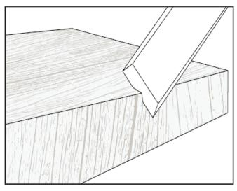
Once you have you chisel sharpened to the desired angle, use a piece of scrap wood and slide the edge of the chisel along the edge of the wood to remove the burr.
