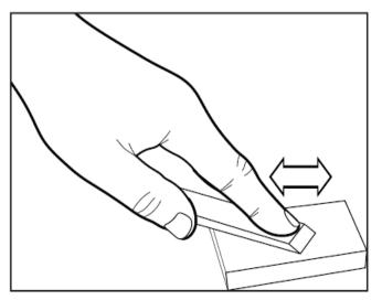
3. Place the back of the chisel (flat side down) against the stone and rub back and forth.
