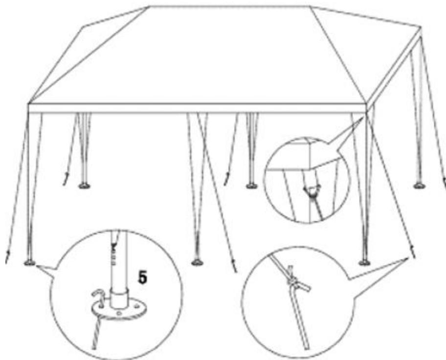
To attach the 6 wall panels, use the Velcro to secure parts onto the main frame.
