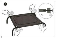
Insert the bolts (D) through the legs to hold the connecting poles in
