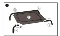
Slide the male leg (B) and the female leg (A) into the longest edges of the mat (E) and join together.
