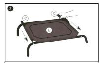
Slide the connecting poles (C) into the shortest edges of the mat.
