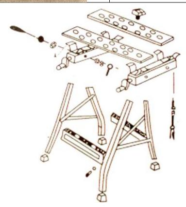
**Step 1:** Firstly, turn 2 metal wood connectors upside down (11) and attach to one slide base (3) using the screws and nut already pre-inserted in the slide base – Please see photos for reference. Repeat this step with the remaining 2 wood connectors and slide base.
