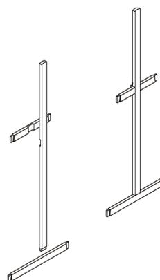
**2.** Align the two Side Frame pieces with in correspondence with the Small Cross Bar and Large Cross Bar ends, and slot into place. The flat end of the Side Frame pieces should be at the bottom, now underneath the Large Cross Bar. Fasten these into place using Large Screws.
