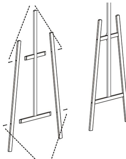
**3.** Using the two Small Screws provided, attach the Hinge to the cross-section between the Small Cross Bar and the Back Frame. This should be done so that the two sides that "stick out" should be vertical. Then, using the Thin Bolt, secure the Support Frame to the Hinge.
