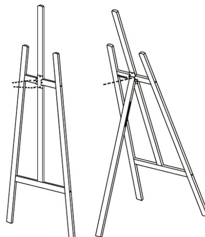
**4.** Using the two Large Bolts provided, attach the Hinge Supports by aligning one of the holes with the slot in the Support Frame, and the other end aligned to the hole just under the cross-section of the Back Frame/Small Cross Bar, on the Back Frame. The gradient of the product can then be adjusted to the user's wish.
