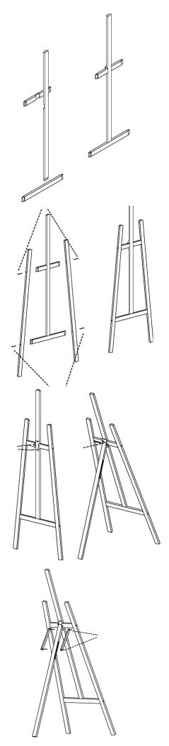
5. Using the four remaining **Bolts**, attach both the **Bottom Bar** and the **Top Bar**. Both of these require connection to a **Bracket** using a **Bolt** through the aligning holes. The bars can be applied at different heights to suit the user's wish.
