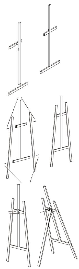
4. Using the two Large Bolts provided, attach the Hinge Supports by aligning one of the holes with the slot in the Support Frame, and the other end aligned to the hole just under the cross-section of the Back Frame/Small Cross Bar, on the Back Frame. The gradient of the product can then be adjusted to the user's wish.
