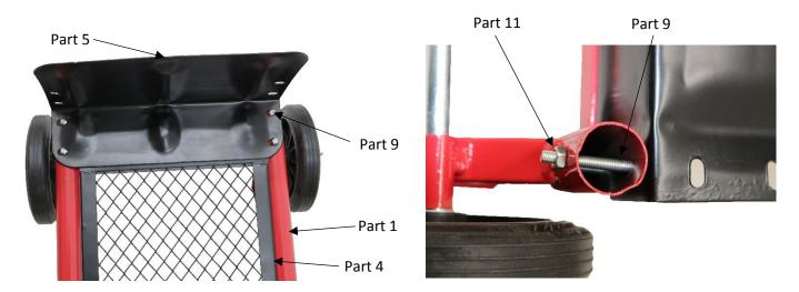
**6.** Place the stopper/platform (part 5) above the mesh (part 4) on the front of the frame (part 1). Push the four bolts (part 9) into the four holes on the stopper/platform (part 5). Secure the stopper/platform (part 5) into place by tightening small nuts (part 11) onto the bolts (part 9). Please see the images above for further detail.
