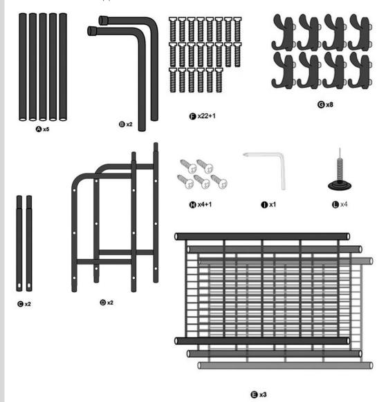
Install from the bottom up. Ensure that all the framework is correctly assembled and aligned before fully tightening the screws. Firstly, insert the larger screws (F) to the support frames (D) and secure these by tightening them to the shelves (E). Repeat with the other 2 shelves. Please note that the support frames are not identical. The screw recesses should be pointing outward. Please see diagram above for guidance.
