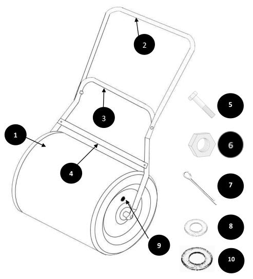
Before commencing, check that you have all the components: roller drum (1); handle (with sponge) (2) bottom section (3); scraper (4); fixings (5, 6, 7, 8).
