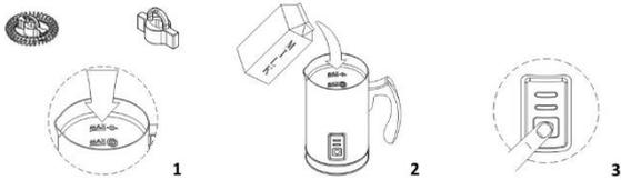
1. Place the milk frother on a flat, level surface. Choose the appropriate whisk, and insert firmly onto the shaft at the base of the jug.
