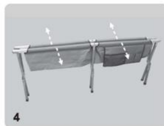
4 Pull both sides apart to open the frame.
