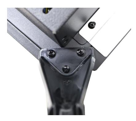
1. Place the electric stove heater (part 1) upside down, making sure to not break the front glass panel. Once done, align the holes in a support leg (part 2) with the holes found in the corners of the bottom of the electric stove heater (part 1). Secure the support leg (part 2) into place using the truss screws (part 3). Repeat this for the remaining corners. Please see the image to the left.
