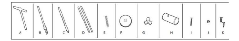
A: T-Shaped Handle B: 3 Prong Tube C: Slotted Ejector Tube D: X2 Ejector Tubes
