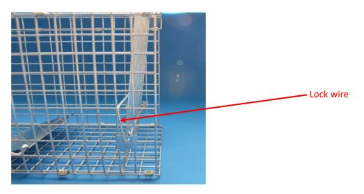
4. Attach the trap hook to the floor plate and then to the U-bend spring clip on the door. Ensure the hook on the spring holds the door open in the cocked position.
