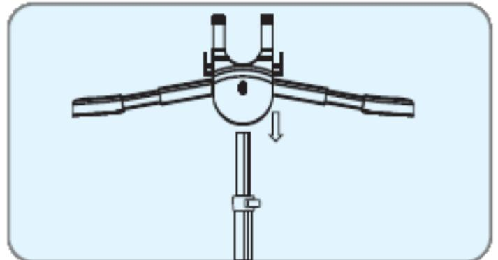
4. Install the hanger onto the support pole, by sliding the hanger onto the top of the pole.
