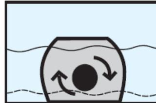
Unscrew the drain valve and drain the residual water from the main body. Tighten the valve after the water has drained.
