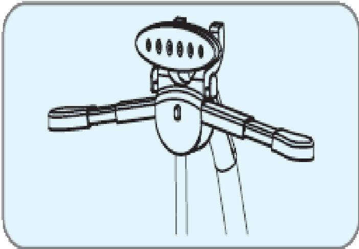
**5. To store the nozzle when not in use, Place the nozzle on the inside of the hanger hook. As shown in the image above.**
