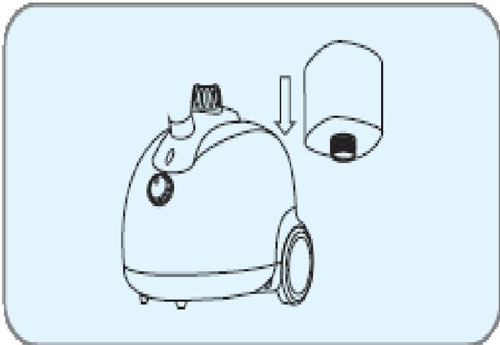
**7. Wipe off any excess water before placing the water tank back into the base.**
