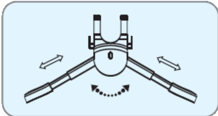
3. To unfold the hanger arms, push the centre button inwards and adjust to the proper position.
