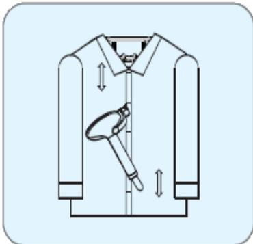
3. If the clothes are covered in dust or hair etc., install the brush onto the ironing head to brush away.
