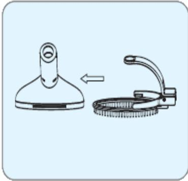
1. Mount the multifunctional brush onto the ironing head.
