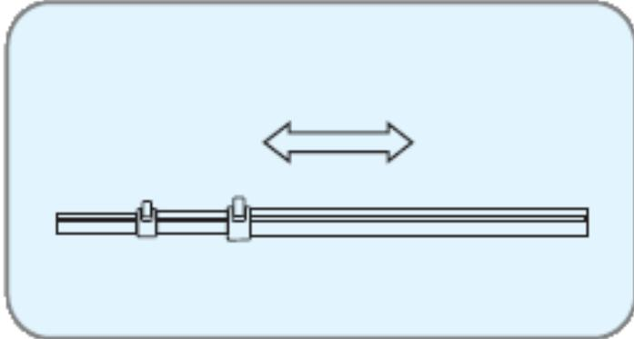
1. Begin by taking the height adjustable support pole and loosen each locking nut. Once adjusted to the desired height, fasten the locking nuts again.
