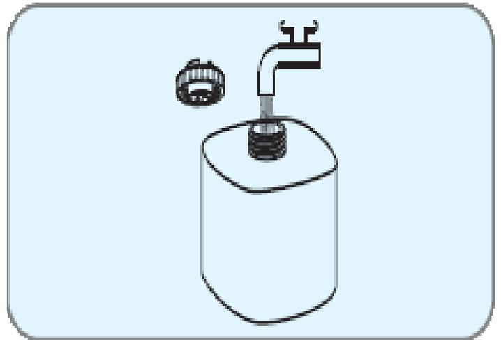
**6. Before plugging the product into the mains, remove the water tank located at the back of the base. Unscrew the tanks lid and add water only, once full screw the lid on firmly.**
