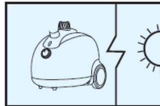
After the water is cleared from the water tank and main body, store the steamer in a warm, dry place.
