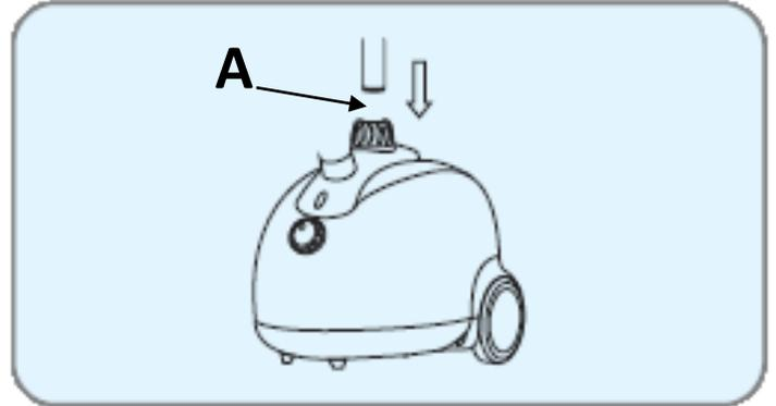
2. Insert the supporting pole into the hole on the top of the steamer. To secure into place tighten the large nut make with an A in the image above.
