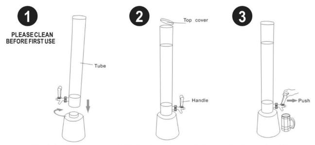
Insert the tube into the top of the base and turn to tighten.
