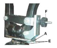
Place the ring (A) onto the hooks (E) and tighten the knob (F) to lock everything together.
