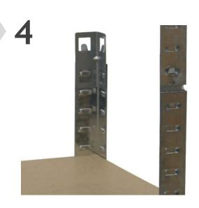
Push a corner extender into each of the exposed corner support bar tops. Once done, slide a corner support bar onto the outside of the corner extender. Make sure this is held securely as this area will be holding the weight of the racking above. Repeat this with the remaining corner support bars.
