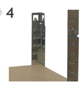
Push a corner extender into each of the exposed corner support bar tops. Once done, slide a corner support bar onto the outside of the corner extender. Make sure this is held securely as this area will be holding the weight of the racking above. Repeat this with the remaining corner support bars.
