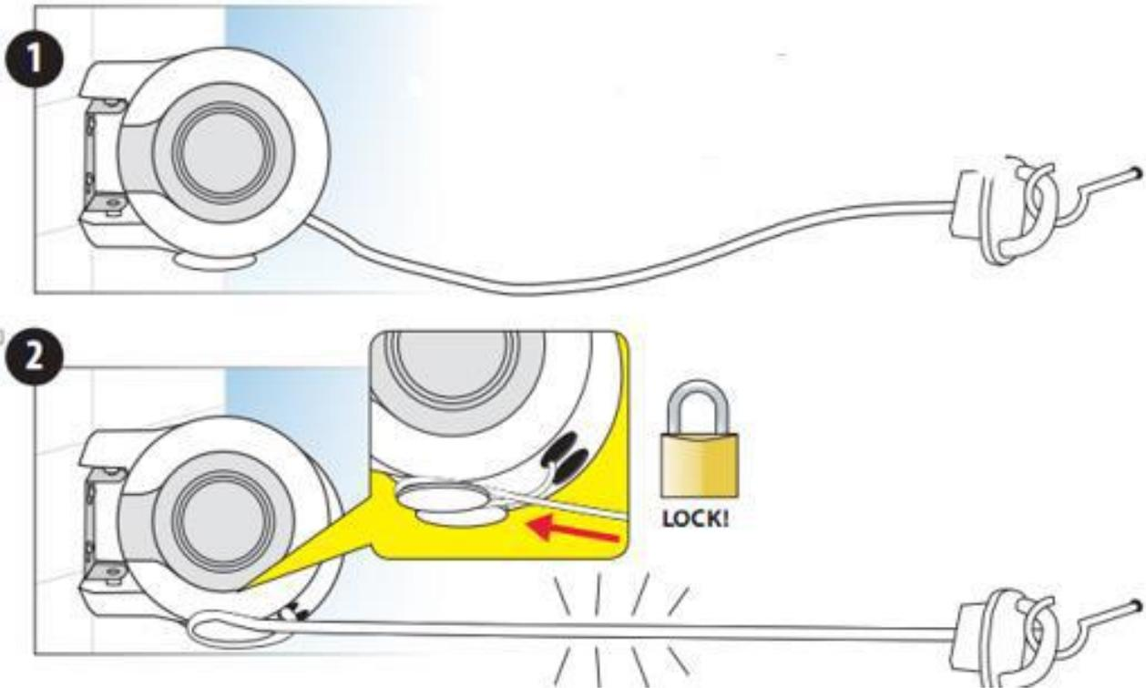
1. After the reel is properly installed, extend the line by pulling on the line hook and fastening to the screw eye hook.
