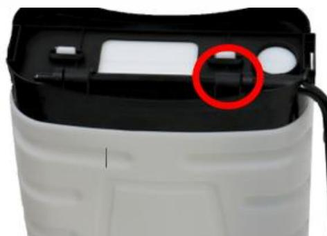
4. The next step is to connect the connecting rod to the pump lever by sliding through the little hole as seen in the photo. Secure in place using a safety pin and washer. Ensure that this is with the smaller end of the connecting rod.
