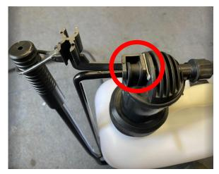
Lastly, just place the filter into the filling point. This prevents anything other than liquid entering the tank. Don't forget to add the pump fastener to the groove in the base of the pump inside the tank. This helps keep it secure.
