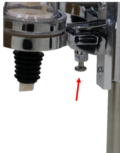
5. Keeping the pin pulled down slot the optic back in so that the optic is correctly orientated (as picture to right) then release the pin and ensure the optic is locked in place.
