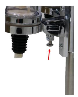
4. Locate the pin next to any of the optics. Then pull the pin down until it stops and pull the optic from its slot.
