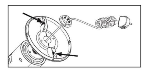
4) Secure the main body and base by turning the adjusting plastic screw nut clockwise.
