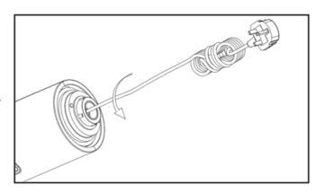
2) Position the base to the main body, ensuring the holes in the two base parts are aligned correctly.
