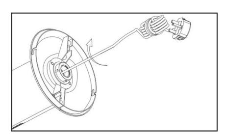
5) Feed the power cable through the slot on the base.
