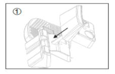
Fix the speedometer onto the loader body with two 5\*14 screws.
