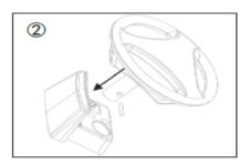
Fix the steering wheel under the front wheel shaft with one 5\*25 screw.
