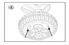
Attach the two front wheels to the front shaft, then put in the front cover, finally put in anti-back ring.
