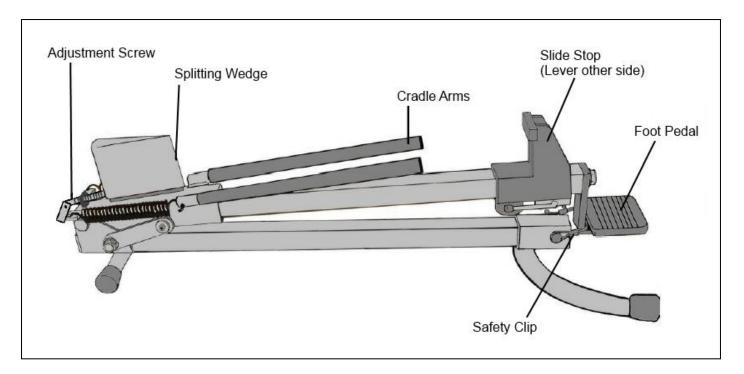
**WARNING!** The foot pedal is under tension. Before removing the safety clip, put your hand on the pedal to prevent it flying up and injuring you.
