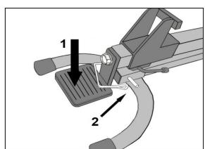
Adjusting the Working Height: Remove the safety clip and adjust the foot pedal height to at least 33cm (13 inches) by screwing the adjustment screw out (anticlockwise) to raise the foot pedal and in (clockwise) to lower the foot pedal.
