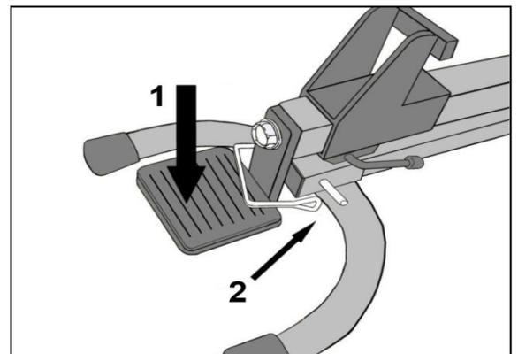
**Adjusting the Working Height:** Remove the safety clip and adjust the foot pedal height to at least 33cm (13 inches) by screwing the adjustment screw out (anticlockwise) to raise the foot pedal and in (clockwise) to lower the foot pedal.
