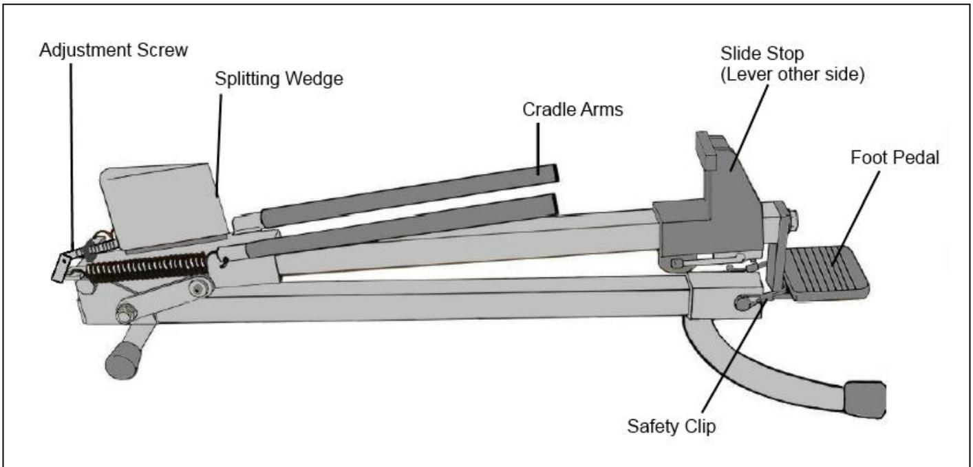
**WARNING!** The foot pedal is under tension. Before removing the safety clip, put your hand on the pedal to prevent it flying up and injuring you.
