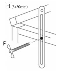
Lastly, attach the lid support arms (E) to either side panel (C1, C2) by using the large H screws (2 X 3x20mm) which are left. Secure these into the lid panel (D), before using the wing nuts to fully attach the support arm (E) to the frame. Again, please see the diagram above for guidance if required.
