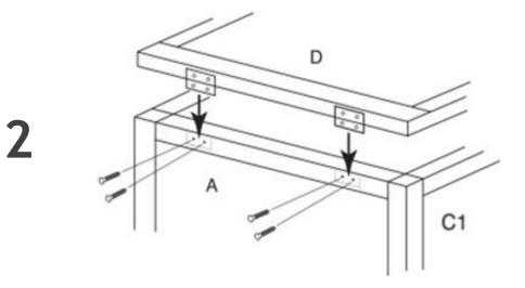
Next assemble the roof/lid panel (D) to the frame built in step 1. Ensuring the hinges (D) attach to the back panel (A). Secure these in place with part I screws (4 X 2.5x10mm). Please see the diagram above to help you.
