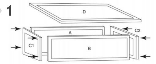
Assemble the back, front and side frames (A, B, C1, C2) using the H screws provided (8 X 3x40mm). Please see the diagram above to help you.
