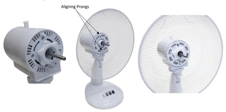
2. Unscrew the back fan-locking nut (part 6). Take the back fan guard (part 4) and slide onto the fan body (part 10). Make sure the two prongs align on the fan body (part 10) with the holes on the back fan guard (part 4). When aligning the back fan guard (part 4) make sure the handle is facing upwards like in the image above. Do not over tighten.
