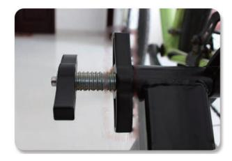
Now you should tighten the magnetic resistor to contact the tyre by again twisting the tyre pressure screw. You should turn it in a clockwise direction. Once it is in contact with the tyre, you can now decide the resistance that you would like to have. The tighter you turn the tyre pressure screw; the more resistance you will feel.
