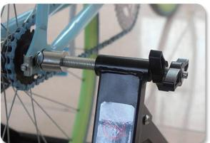
Once the left and right sides are locked well onto the rear axle, you can rotate the locking handles towards the bike trainer. Once this is tightened, the handles will not need to be adjusted any further.
