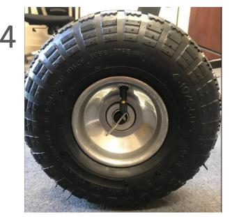
Finally, slide each wheel (7) onto the front axis and fasten them in place using the safety pins (11) through the pre made holes. Please see photo for reference.
