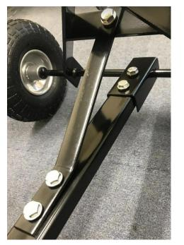
Firstly, attach the middle support bar (3) to the bottom of the front axle (1) using 2 small nuts and bolts (9). Please see photo for guidance. Then, attach the front axle support (5), to the middle support bar using the 2 remaining small nuts and bolts. Secure tightly. Lastly, attach the other end of the front axle support to the middle section of the front axle using the 1 medium nut and bolt (10) provided. Secure tightly and move on to step 2.
