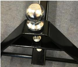
For step 3, simply securely attach the tow bar (6) onto the top of the front axle (1). Please see photo for help and move onto part 4 on the next page.
