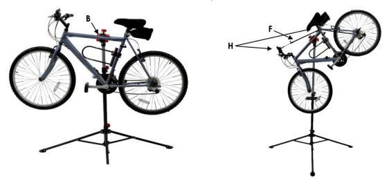
3. To attach the Front Wheel Stabiliser (F) to the bike, firstly attach the end of one grip (H) to the Front Wheel stabiliser. Next, tightly attach round one of the bike's handle bars and re-attach to the Front Wheel stabiliser by pushing through one of the remaining holes. Repeat this with the other grip (H) and the Adjustable Stand Pole (C) so that it is securely attached to both bike and stand.
