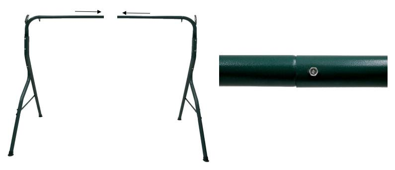
**6.** Slide both supporting leg sections together. Please see the image above. This part may require two people. Take a medium bolt (part 19) and push it through both joint bars, holding them in place. Secure these by using a small nut (part 20). Secure tightly, but do not overtighten, to ensure the product is stable.
