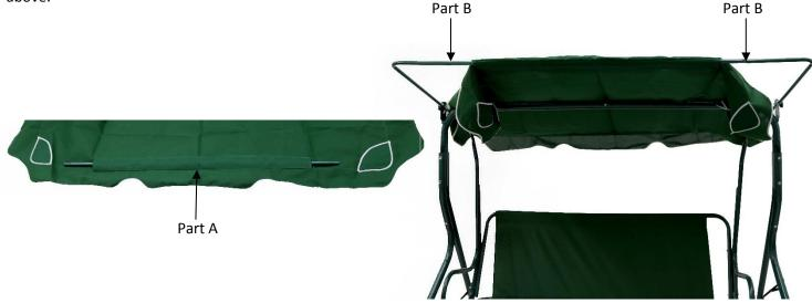
**11.** Take one of the canopy front or back poles (part 11) and slide the pole through the canopy (part 12), ensuring it goes all the way through (part A). Now use repeat this process for the opposite side. After ensuring the canopy is on correctly, slide both parts into the canopy sides and make sure that they are locked in place in both the front and back (part B). Please see the images above.
