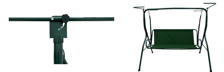
**10.** Secure the canopy side (part 10) onto the top of the support frame using an adjustment screw (part 23) and a small bolt (part 21). On the outer side of the support frame, ensure they stay in place by securing the adjustable screw (part 23) with a wingnut (part 24). For the small bolt (part 21) it should be secured with a small nut (part 20). Please see the images above.
