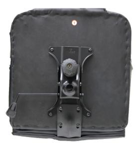
**4.** To attach the chair back support to the chair seat, align the holes on the metallic section of the chair back support with the holes on the adjustment platform. Once done, secure the chair back support in place with the regular screws (M6X30). Make sure the screws are tightened correctly. Please see the image to the left.
