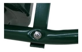
**3.** Slide the roller handle on the inside of the roller beams, ensuring that the roller handle is directly against the inside of the roller beams. Once done, push a bolt through each hole, ensuring it goes through both parts. Once done, tighten a nut onto the bolt. Do not overtighten as this may cause the bolt to bend. After this, repeat this step to fully attach the handle.
